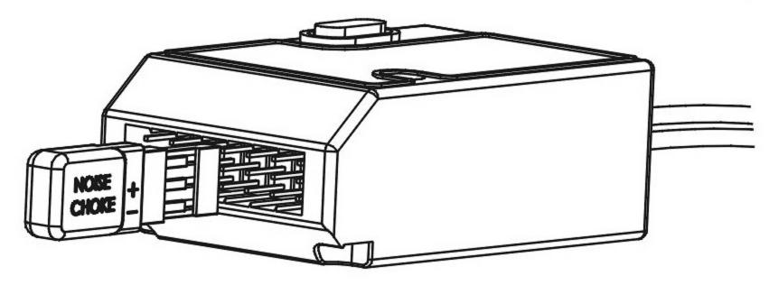
Please insert the noise choke to any un-use channel of the receiver. 插入接收器任一未使用的通道。
