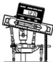
Stick position at high/Throttle 100%/Pitch+12° 搖桿高速/油門100%/Pitch+12°
