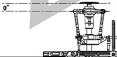
Stick position at middle/Throttle 90%/Pitch 0° 搖桿中速/油門90%/Pitch 0°
